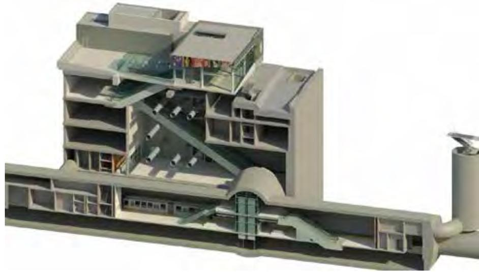
FIGURE 4: Longitudinal Cut-Away along completed Chinatown Station
