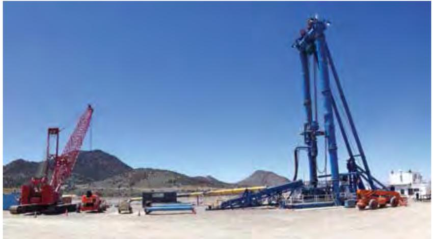
Frontier-Kemper makes history again with a new, US record for the largest, single-pass, full-face, Blind-Drilled Shaft. This drilling feat was accomplished on February 20, 2014 with the completion of the South Vent Raise Shaft at Barrick Gold's, Cortez Mine in Crescent Valley, Nevada. The Blind Bore Drilling Team was able to successfully drill a 16-ft. diameter shaft at 1,634 ft. deep.
